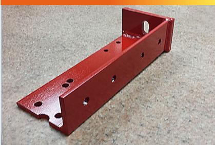
One of the many different products manufactured at Valco Industries are mounting supports for diesel fire pump engines that are used in the fire protection industry. These heavy weldments combine steel bases and structural carbon steel angles:
