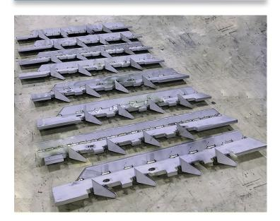
Valco recently had an opportunity to shine by manufacturing Paddle Bars for a Springfield manufacturer of processing equipment. We manufactured 8 different paddle bars that work together to extrude corn in the manufacture of ethanol. These paddles were challenging in both tolerance and delivery. Valco delivered the 9 units in 3 working days after receipt of drawings. The nearly 20 lb. pieces all weighed within 1/2 oz. of each other per drawing requirements.
