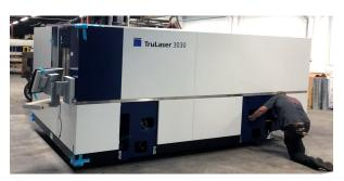
Both Trumpf 3030 TruLasers now sit in a reconditioned area of our facility, positioned as mirror images for more efficient material handling. Both machines are equipped with LiftMaster Compact loading/unloading systems which will be accessible from a central area.
